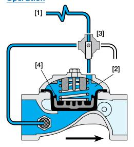
Hydraulic Command [1] is applied to the Control Chamber [2] through the Manual Selector [3]. This creates superior closing force that moves the Diaphragm Assembly [4] to a closed position. 16 Discharging pressure from the control chamber, by turning the manual selector, causes the line pressure acting on the lower side of the diaphragm assembly to move the Valve to an open position.
