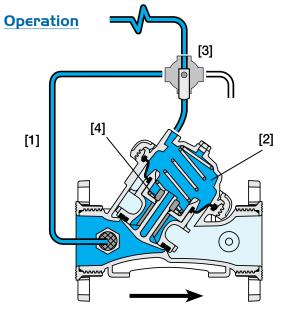
Line Pressure [1] is applied to the Control Chamber [2] through the Manual Selector [3]. This creates superior closing force that moves the Diaphragm Assembly [4] toward a closed position.
